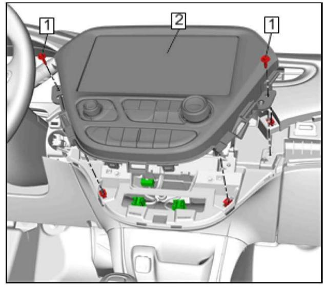
4. K73 Telematics Communication Interface Control Module Removal.
